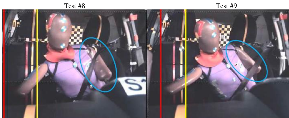
Figure 21: With and without pretensioning – belt to arm interaction
