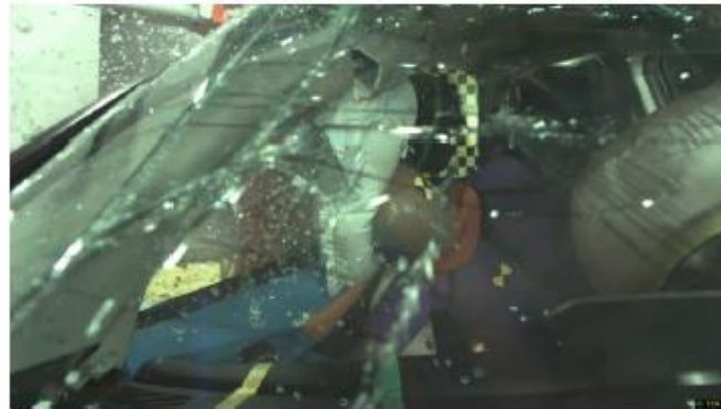
Figure 10: Oblique pole impact - 36km/h
