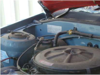
Mid-1980s: Stiff firewall and sides of engine bay supporting edge of bonnet. Minimal clearance between suspension tower/air cleaner and bonnet.
