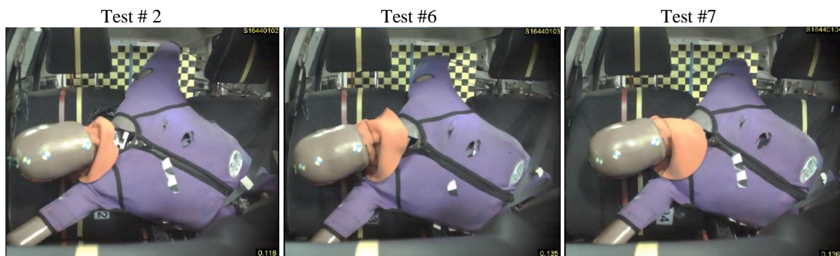
Figure 18: Modified APROSYS pulse vs 36km/h pulse vs 32km/h pulse - max head excursion
