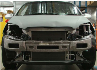
Lower support in position to keep leg from bending under car and energy absorbing foam to protect the knee.
